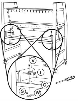
Step 8: Install the power tray back panel (H) with 4 screws (S), using a screw driver.
