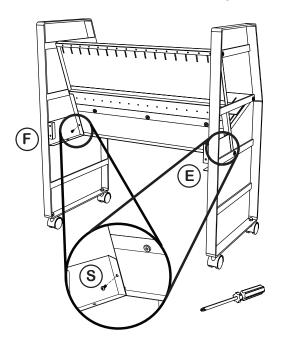
Step 6: Attach the bottom power tray panel (G) with 2 screws (S) from below, using a screw driver. Attach the 2 power strip brackets
