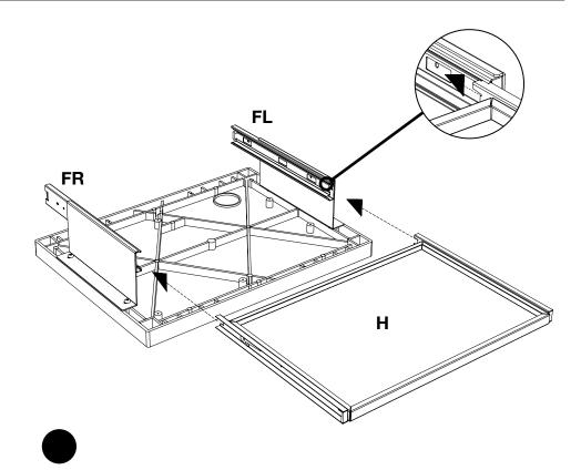
Take the top shelf of your plastic cart and lay it flat. Collect parts: **FL**, **FR** & **A**. Align **FR** & **FL** to the outer holes at the top of the shelf. Take screw **A** and fasten with a screwdriver, do not tighten fully until keyboard is attached.
