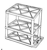
Position bottom shelf, ribbed side up, over the 4 legs and insert leg posts into legs. Using a rubber mallet, firmly hammer bottom shelf into legs until all 4 legs are seated (flush) against the surfaces of both shelves.
