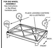
Push the four casters firmly into the holes in each corner of the bottom shelf. Important: Casters must be fully seated. Tap firmly with rubber mallet to properly seat casters. Turn your LP table right side up. It is now ready for use.
