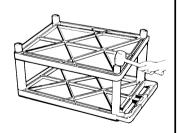
Position center shelf (with 8 leg posts) ribbed side up, over the 4 legs and insert leg posts into legs. Using a rubber mallet, firmly hammer center shelf into legs until all 4 legs are seated (flush) against the surfaces of both shelves.
