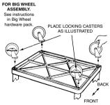
Push the four casters firmly into the holes in each corner of the bottom shelf. Important: Casters must be fully seated. Tap firmly with rubber mallet to properly seat casters. Turn your LP table right side up. It is now ready for
