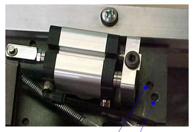
Mount the air cylinders in the top inside holes / for C-size blade configuration.
