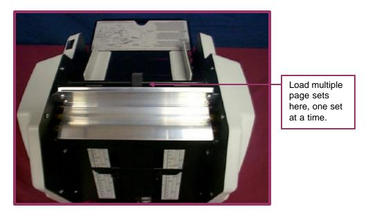
NOTE: Your unit can run stapled sets, but they must be stapled parallel to the top edge, and the staple must be centered. Also, when hand feeding sets into the machine make sure that you use the engaging clip to hold the feed table in the down position. If this were not done, it could cause premature wear of the feed tire.
