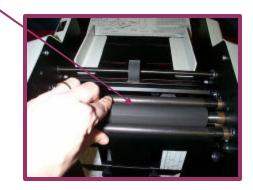
3. If necessary, remove each of the folding tables by disengaging off of mounting pin and lowering down until it separates.
