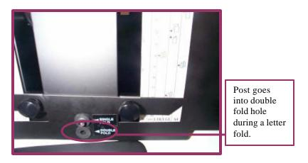
NOTE: When doing two folds, make sure that both folding tables are pointing to an identical icon.
