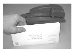
**Step 1.** Prepare up to 10 standard envelopes to be opened by tapping the top sealed flap side down firmly on desktop several times. This will cause the envelope contents to slide to the opposite side of that to be opened.
