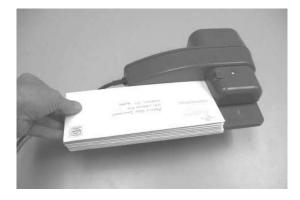
**Step 2.** Place up to 10 prepared envelopes onto the feed tray with the bottom edges of the envelopes back against the opener housing and also against the top cover that contains the **START** button.
