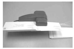
**Step 4.** Depending on the condition of the envelope edges and flatness, the entire stack should automatically feed until the stack is completed. However, under previously mentioned conditions of the envelopes, you can depress the **START** button to begin feeding again if it hesitated and did not complete the stack.
