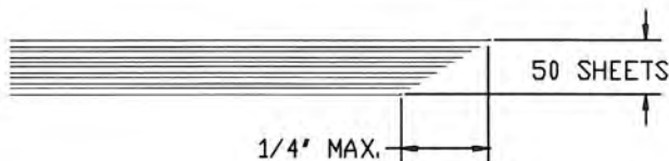
Side view of fanned paper Fan paper no more the 1/4”(6mm) per 50 sheets
