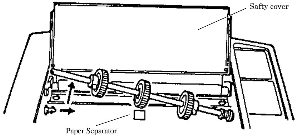
Grasp the paper separator (with plastic part) at both ends and pull it out.
