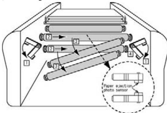
Remove the upper roller in the order of **1** to **3**, and then remove the lower roller.
