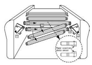
Remove the upper roller in the order of  $\begin{bmatrix} 1 \end{bmatrix}$  to  $\begin{bmatrix} 3 \end{bmatrix}$ , and then remove the lower roller.
