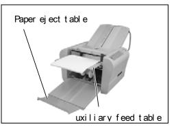
Pull the paper eject table out and lift the auxiliary feed table into position.
