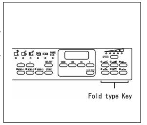
Select the memory key in which the fold will be input. Hold down the STORE key and release immediately when you hear a beep.
