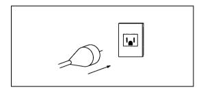
Insert the power cord into the inlet.
