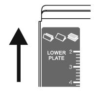
When the 2nd fold plate(short plate) put in , Please see clearly the labels at both ends as shown.
