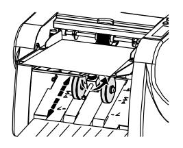
Setting the paper delivery roller according to folding patterns.
