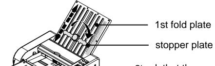
Check that the paper has been folded correctly and if necessary adjust the stopper plate on the 1st fold plate and/or 2nd fold plate. As soon as the 1st fold plate is correct, adjust the 2nd fold.
