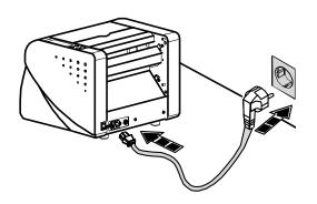
Connect the power cord to a single phase socket . 120V/4A
