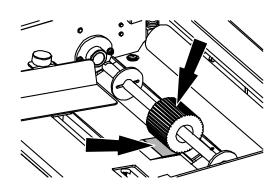
Wipe the surface on the feeding rollers with MBM roller cleaner.
