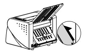
Check that the 2nd fold plate is in the correct position.
