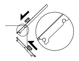
Insert the 1st fold plate(long plate) into the studs (A) and (B) and lock into position.
