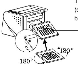
Turn the 2nd fold plate 180 degrees (script is in reversed position) and put back into the machine.
