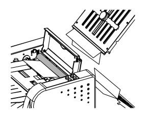
Remove both fold plates and any paper debris.
