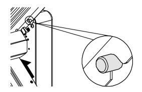
Fix the fold plate tightly (the hook of the fold plate click on the supportive).
