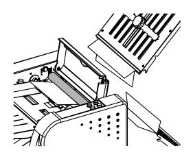
Remove both fold plates and any paper debris.
