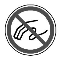
Do not touch or insert foreign objects into any rotating part during operation.
