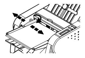
Move the paper guides to the edge of the paper. Tighten the screws.
