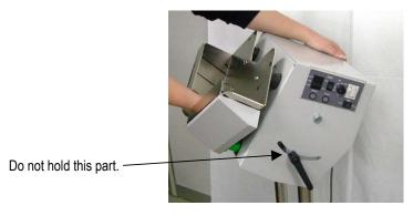
• In general, for thick paper, the tilting angle is adjusted vertically and for thin paper, it is adjusted horizontally.
