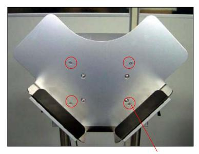
Fasten the countersunk screws at the four locations.
