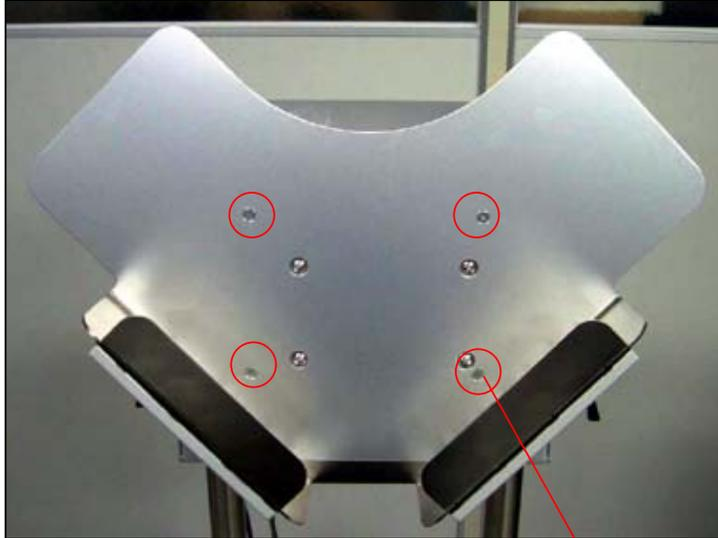
Fasten the countersunk screws at the four locations.
