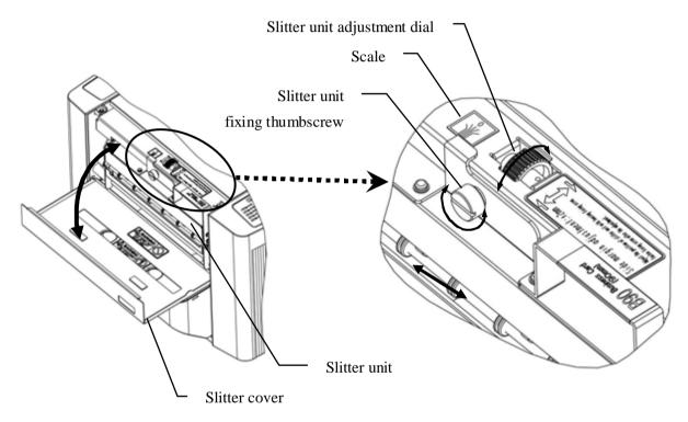
\* After completing the adjustment, securely tighten the slitter unit fixing thumbscrew.
