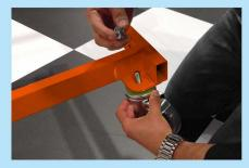
Begin bolting wheels onto base frame making sure each wheel is tight
