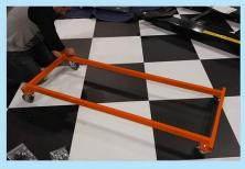
4. Lock wheels into place for easier assembly of rest of rack
