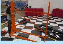
Tighten all bolts and nuts on cross braces and horizontal beams and then double check all rack sides and wheels for tightness.
