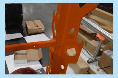
6. Before tightening all the rack side bolts, begin adding cross beams and braces.
