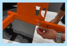
5. Using the longer bolts and nuts, start adding rack sides
