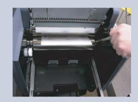
You can check the jam within the press roller by sliding out the folding unit. Use the jam removal tool which is attached inside of the machine to remove the jam.
