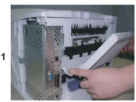
Press with your finger to remove the back cover of the priner.
