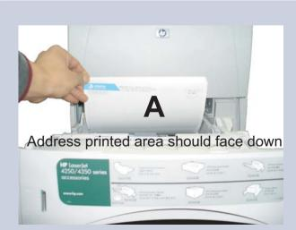
Make sure that the papers are loaded properly in the printer.
