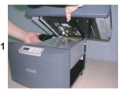
Attach the interface unit onto the main body.
