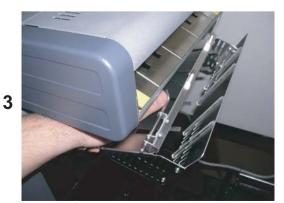
Push the hinge and fix the interface guide like the picture.
