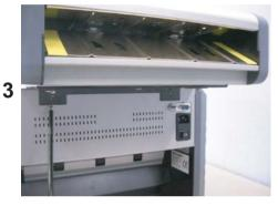
Fix the interface unit onto the main body.
