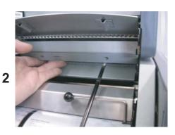
Connect the main guide and the interface guide together.
