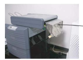
**INTERFACE GUIDE** Interface guide enhances the infeed process of each processed forms.
