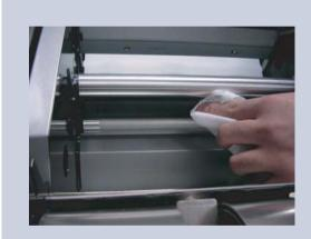
You will be able to see the folding roller when you release the bottom lever of the folding unit.
