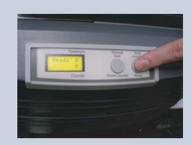
Beeping noise indicates a paper jam within the mailfinisher. After removing the jammed paper, press the RESET button. If the machine is still making the beeping noise, please check for any other paper jams.
