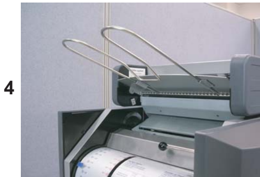
4 Assemble the upper tray guide.
