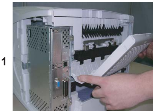
1 Press with your finger to remove the back cover of the printer.
