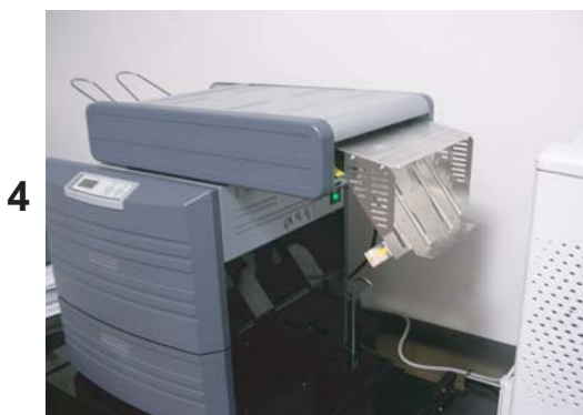
4 Lift up the interface guide.
