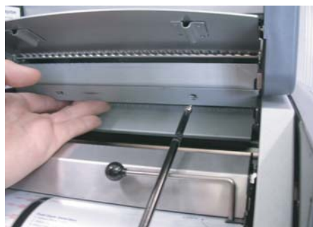
Please check the connection between the main guide and the interface guide.
