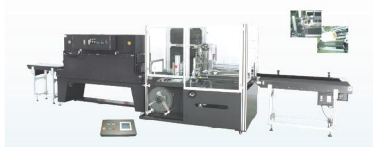
The picture above displays our side seal system with high speed tunnel PPG 1808-72 and optimal in & out-feed conveyors
