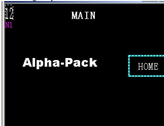
The numbers in the left corner of the screen indicates the RWI No. (For different job parameter easy recall)
