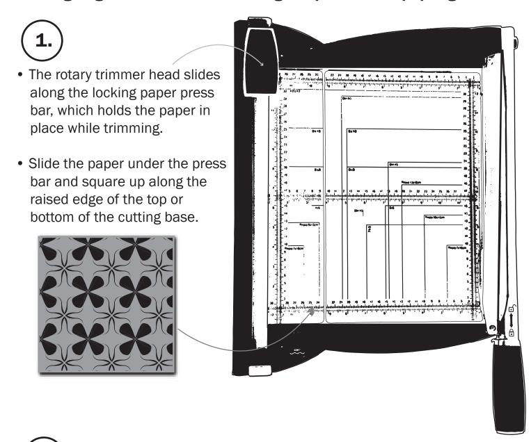
· Lock the press bar by pushing down on the locking mechanism at each end of the cutting rail; they will click into place.
