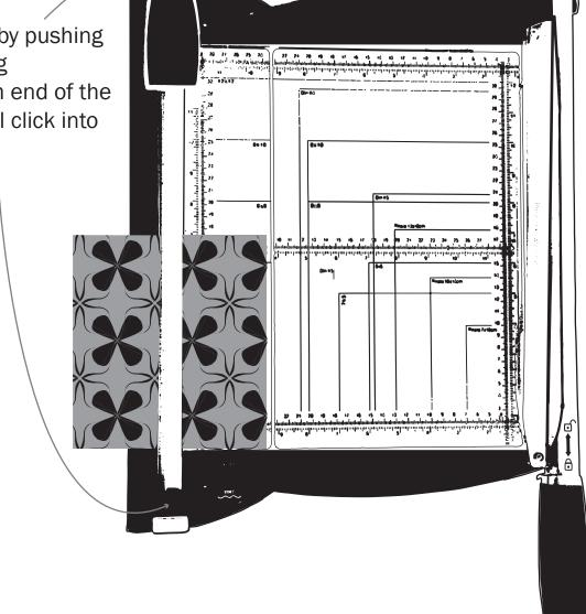
· Slide the cutting head to either the top or bottom of the cutting rail, press down on the cutting head to engage the blade, and slide the cutting head along the cutting guide, while applying pressure evenly.
