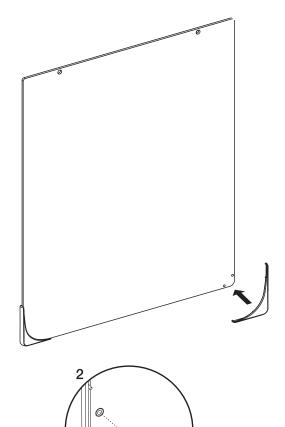
2. Attach each corner cap with (2) no. 6 x 1/4" screws.
