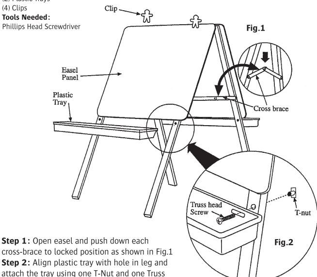
(Note: Extra holes are provided in the legs for raising and lowering easel panel and tray.) **Step 3:** Attach clips to top of easel panel as
