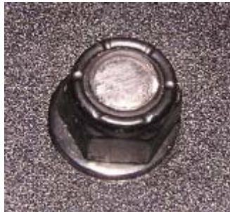
Figure 6: Nylock nut thread position – flush / flat at top of nut - Critical
