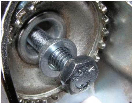
Figure 4/5: Using hardware supplied, secure caster frame to cart
