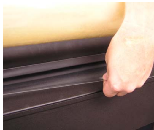
Guide film out the back of the machine
