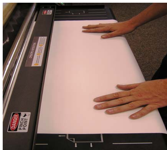
Load item under the paddle, squarely to film
