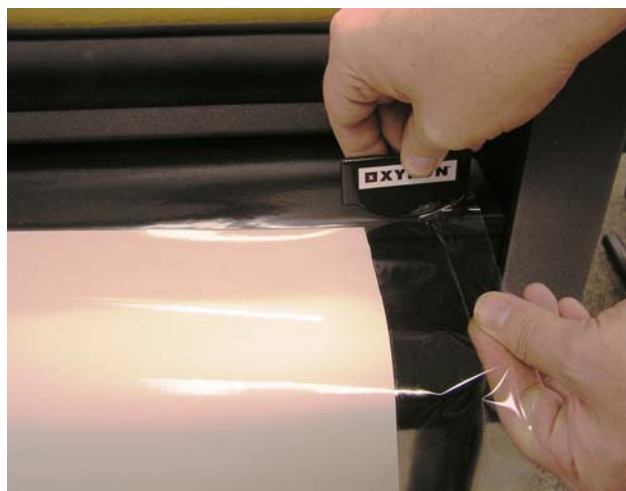
Apply tension to film when cutting
