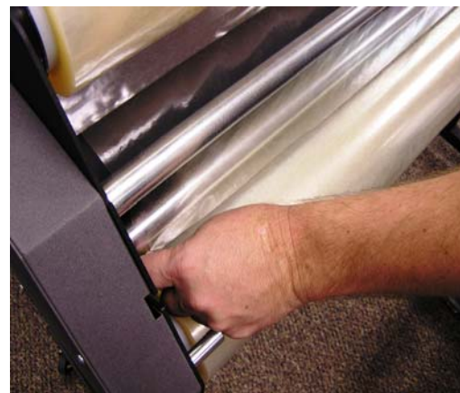
Tacking laminate from top roll to exposed adhesive on bottom roll
